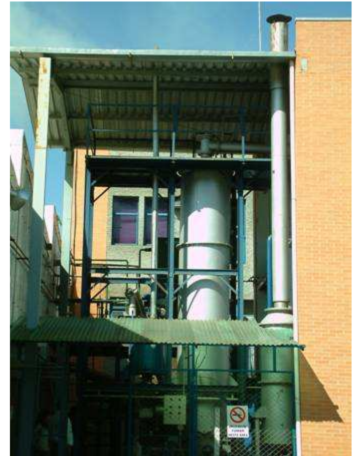
Circulating Fluidised Bed with Tar Cracker
